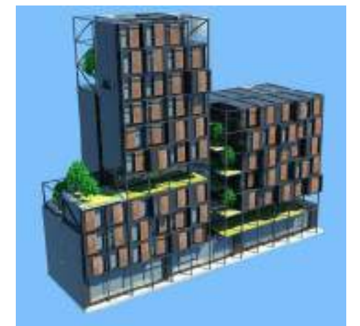
THE ROOMS, ASSEMBLED ELSEWHERE AT THE SAME TIME AS THE EXO-SKELETON IS BUILT, ARE INSERTED
